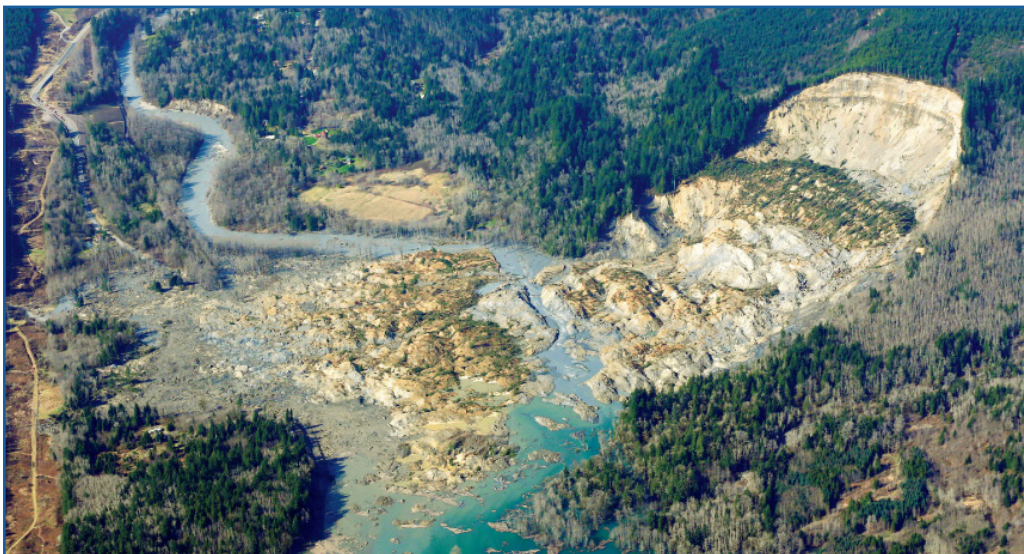
An aerial photograph of the now familiar Oso Landslide, which contained approximately 5 million cubic meters of sediment and temporarily blocked the Stillaguamish River. Seismic signals from the slide were detected up to 170 miles from the slide location. Dave Montgomery was part of the field team that collected data immediately following the event.
