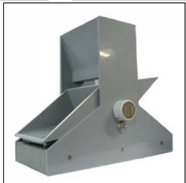
Figure 2. 0.5 L/tip tipping bucket flow gauge measurement
